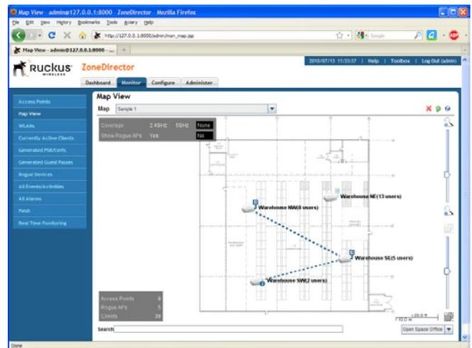
Ruckus Smart Mesh Network is managed centrally from the Ruckus ZoneDirector WLAN controller. Powerful mapping and management tools allow a complete view of the entire Smart Mesh Network, including connections within the mesh, associated mesh clients and other unique controls.
