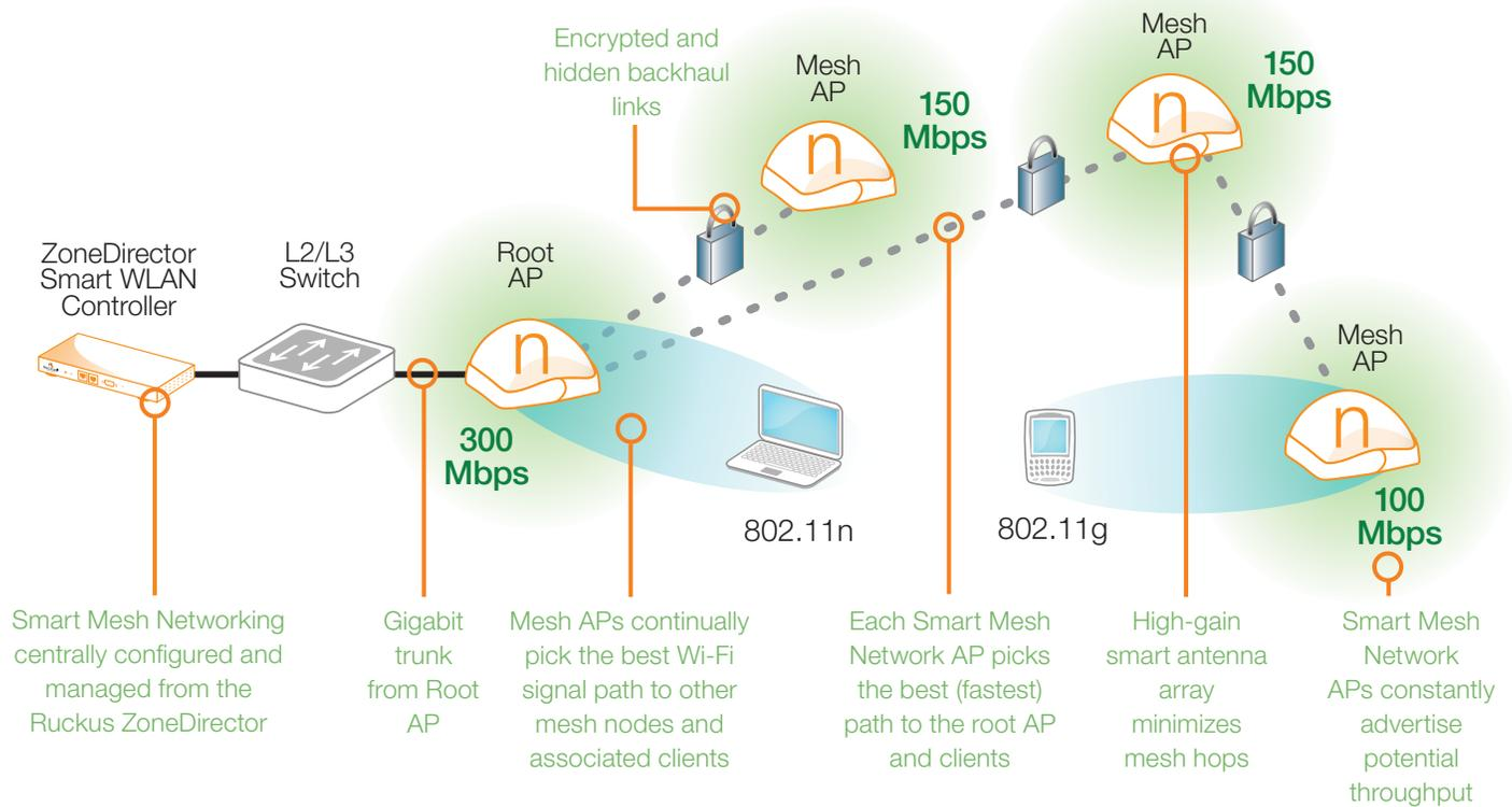
Smart Mesh Networking extends Ruckus Smart Wi-Fi technology to create a new class of reliable and high-performance wireless LANs that are self-organizing, self-optimizing and self-healing. It is the first Wi-Fi meshing approach that combines high-gain smart antenna arrays, sophisticated RF routing and centralized management with a single WLAN system.
