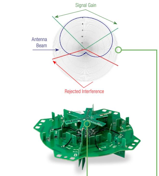
Each Smart Mesh Network AP integrates a patented Ruckus smart antenna array with up to nine high-gain vertically-polarized, and up to nine horizontally-polarized antenna elements. This enables up to 4224 potential antenna combinations and up to 9 dBi gain and 17 dB interference rejection, thereby delivering unprecedented range extension and signal reliability.
