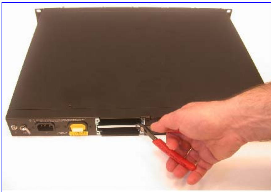
Figure 5-7: Cutting Metal Strip
