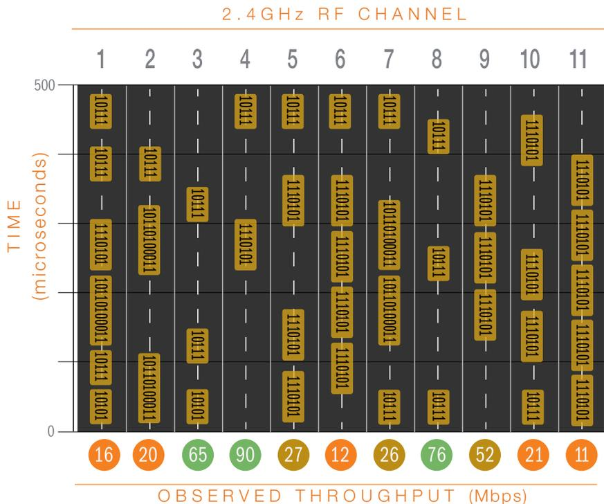
Competitive approaches to RF channel selection go off-channel to passively listen for beacons, CRC errors and other metrics at a given moment in time. In contrast, ChannelFly constantly learns about each channel's capacity using actual activity on across all channels within the 2.4 and 5GHz bands. With this information, ChannelFly builds a statistical model over time to determine what channel will yield the greatest capacity for clients.
