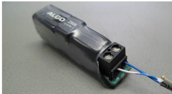
*Note: The pin polarity/placement varies between devices. Ensure correct polarity is used with each device.*
