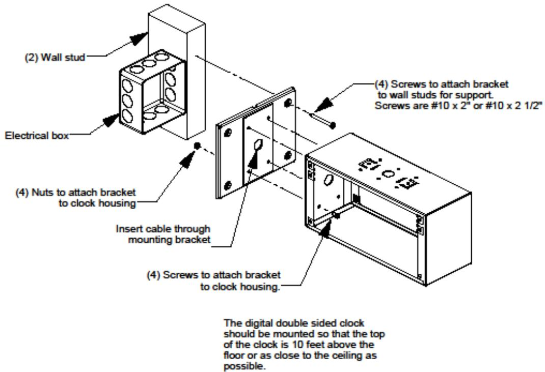
Figure 2. IP Digital Double Sided Clock Wall Mount Diagram
