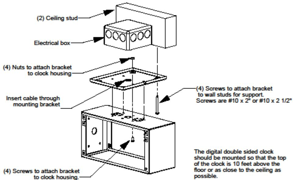
Figure 3. IP Double Sided Clock Ceiling Mount Diagram
