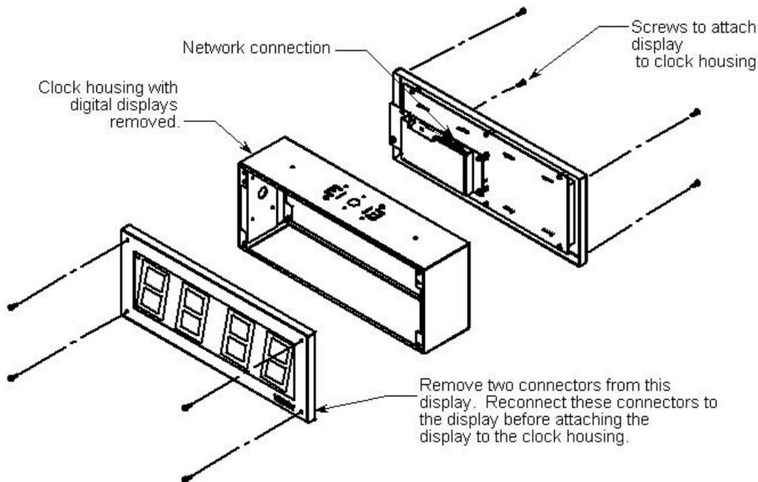
**Figure 1. IP Digital Double Sided Clock Wiring and Display Diagram**
