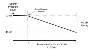
If the reverb time is higher than half of a second in a space, another calculation can be applied for room treatment. Take the square footage of the floor of the room with an average ceiling height. Forty percent of that square footage should be the general square footage of treatment or non-hard surfaces in the space. There are many manufacturers of acoustic paneling, ceiling baffles, etc., that can be placed on the wall to mitigate
