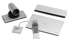
**Cisco SX20 with 12x Camera:** Turn any flat panel display into a flexible, powerful and sleek TelePresence system with high definition video quality, multiparty conferencing and a 12x zoom HD camera.
