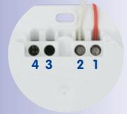
5. **Outputs of power supply unit to screw terminals 3 and 4:** If, instead of a PoE switch/injector, a DC power supply unit (48–57 V) is used to supply power, it is connected to one of the two Mx2wire+ units. See the description for alternative connection options in Section 3.2.
