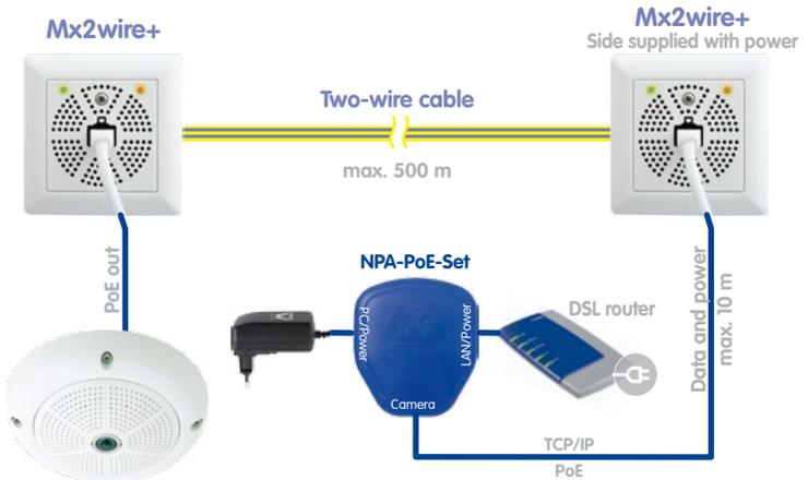
The NPA-PoE set (pictured here) or the weatherproof NPA box (not pictured here, available in 2012) are suited for standard PoE power supply according to IEEE 802.3af
