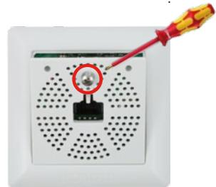
Now remove the attached frame from the circuit board. Please note that you will need the stainless steel screw in the front panel again later.
