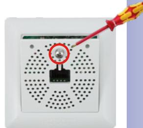
2. Using a small screwdriver, switch the rotary switch on the Mx2wire+ connected to the injector/switch from position 3 to position 4 (see figure). This setting corresponds to the PoE classes 3 and 4 of the injector/switch used.
