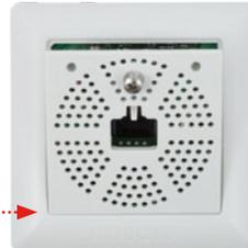
8. **Screw the panel on tightly:** Secure the front panel using the panel's stainless steel screw. Continue with Section 3 (Operation).
