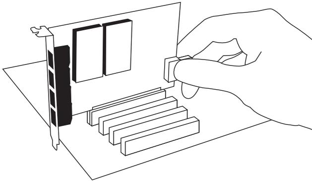
**Figure 6: Connect Power for FXS Modules**
