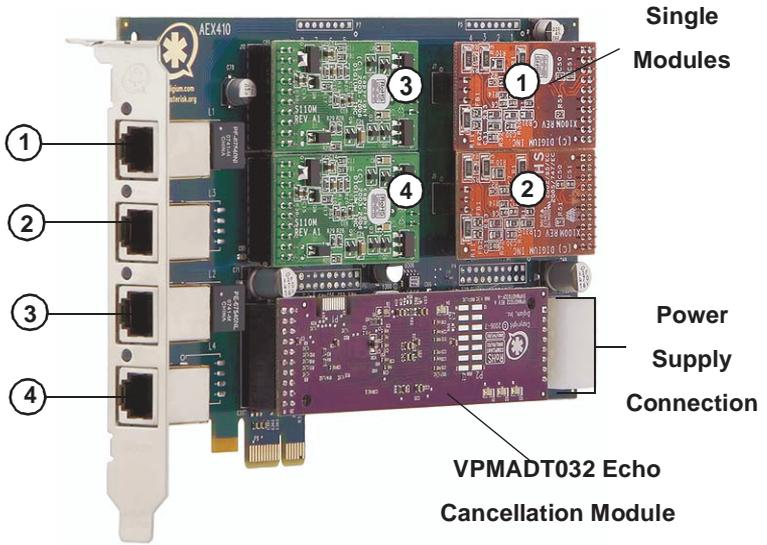
Figure 3: AEX410 Card with Four Single Modules
