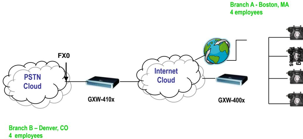
In this diagram, configure the SIP Server field to be the IP Address of the other gateway (i.e. configure IP address of FXS gateway to be SIP Server of GXW410x and vice versa). Please be sure you set SIP Registration to No.
