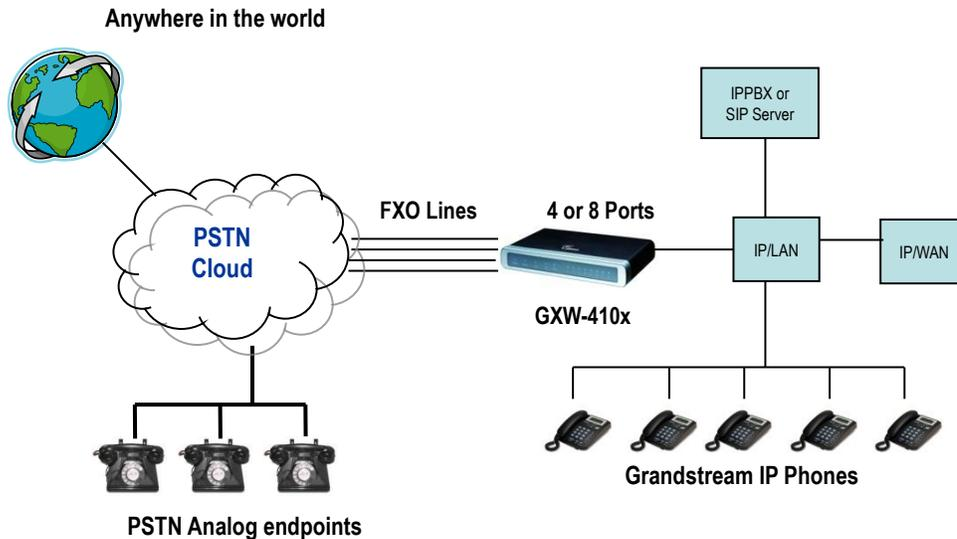
For incoming calls from the PSTN analog endpoints to the GXW410x, the device will auto forward each call to a configured IP extension. The SIP Server can then route the call based on its own configuration or IVR system.
