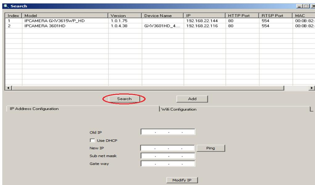
5. Double click the column of the detected camera, the browser will automatically open and link to the device IP and the web configuration page.
