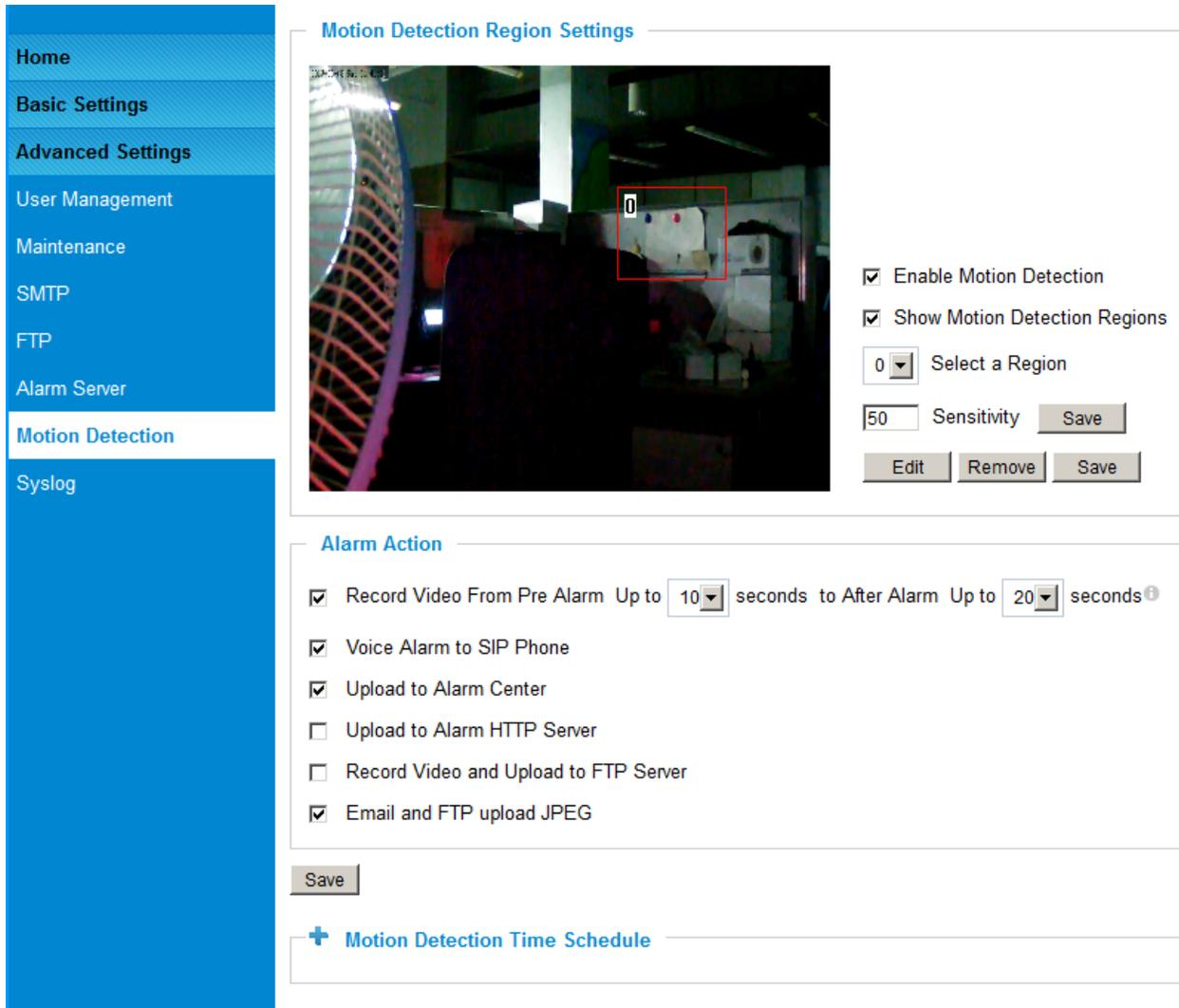
Figure 15-1: Motion Detection Configuration Page
