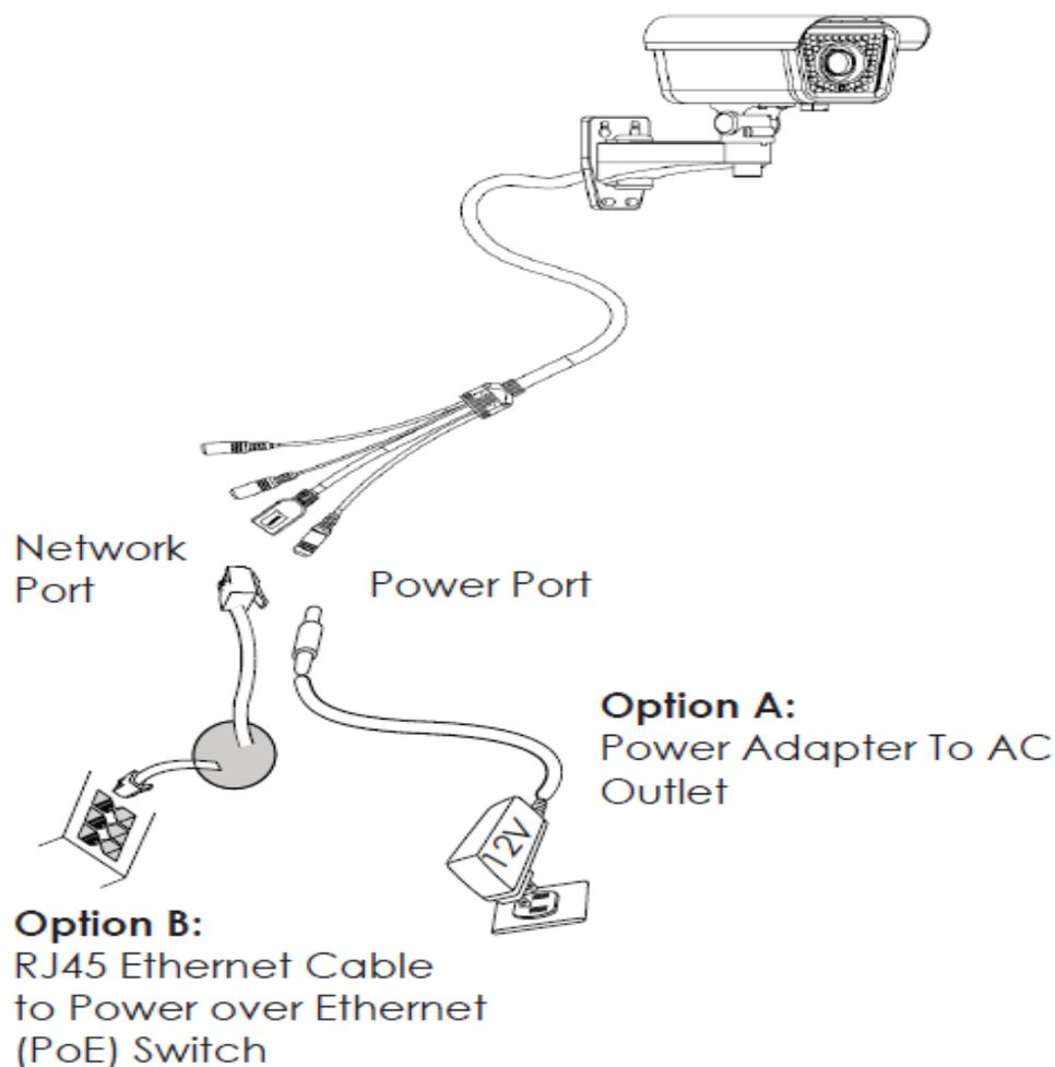
**NOTE:** Choose Option A if using the power supply; or choose Option B if using a Power over Ethernet (PoE) switch.
