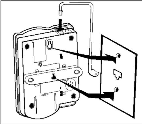
Fig. 6 - Wall mounting installation.
