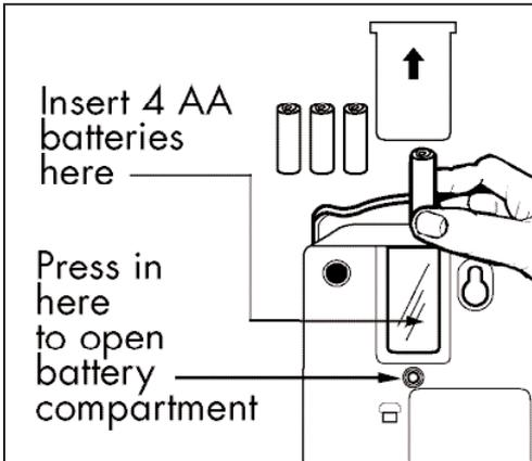
Fig. 7 - Battery installation
