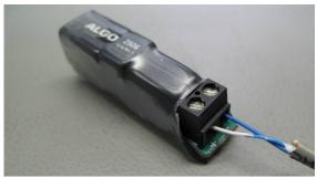
2. As per the table below, connect the wires from the 2506 to the relay input (speaker output on 8180) on the device of choice:
