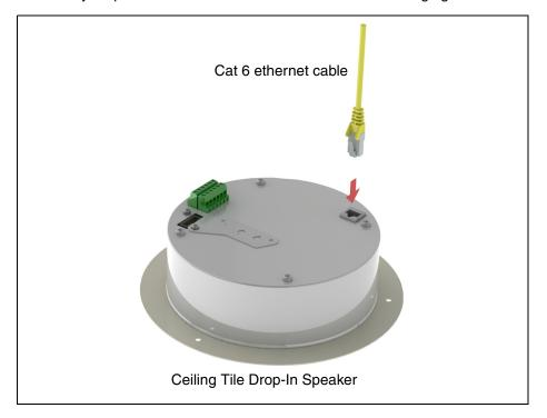
3.2. The IP addressing mode is set to DHCP on default. After 27 seconds, the speaker will beep to indicate initialization.
