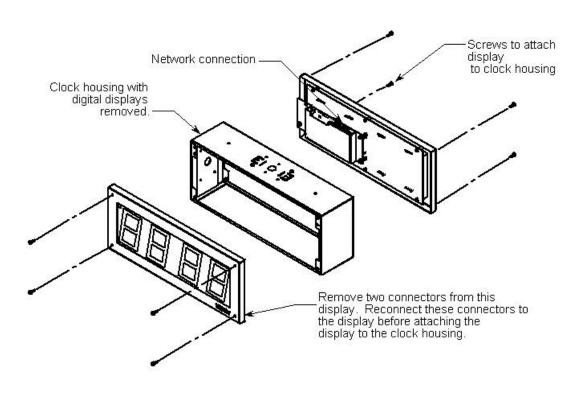
Figure 1. IP Digital Double Sided Clock Wiring and Display Diagram
