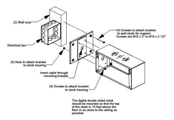
Figure 2. IP Digital Double Sided Clock Wall Mount Diagram
