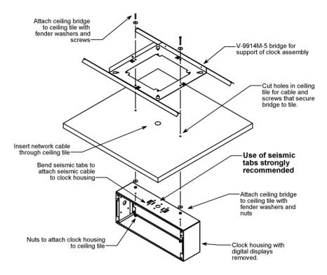
Figure 4. IP Digital Double Sided Clock Ceiling Mount with Optional Bridge Diagram (for D440ADS, D625ADS, D640ADS only) (not for D425ADS)
