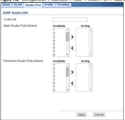
Figure 140 Configuration > Multicast > IGMP > Router Port > Add/Modify
