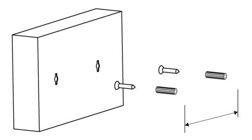
The Switch should be wall-mounted horizontally. The Switch's side panels with ventilation slots should not be facing up or down as this position is less safe.
