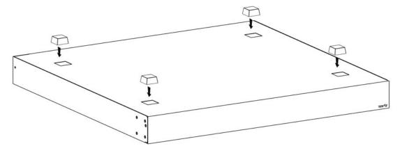
Note: Do NOT block the ventilation holes. Leave space between devices when stacking.
