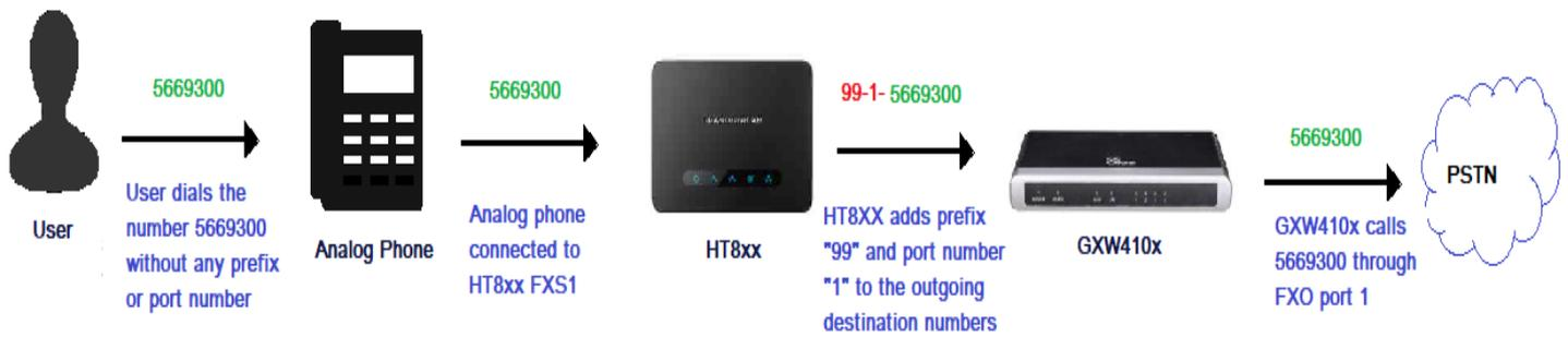
**Figure 15: Port-To-Port Mapping call flow**
