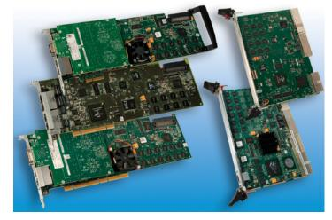
tone detection/generation, echo cancellation, and voice compression, as well as trunking, fax, conferencing, and VoIP functions in a single PCI, CompactPCI, or PCI Express slot. The universal port feature eliminates the need to use multiple specialized boards, provides easy access to all supported features, and significantly reduces the time spent on configuration and development.
