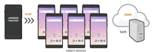
Versity devices are factory-loaded with the SAM client and other Spectralink applications. After the Android Master bump, Versity receives network information from the EMM and then establishes a secure tunnel with the SAM server. Essential feature settings are provided by SAM and Versity is now fully functional.
