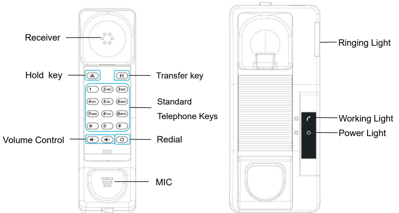
The above picture shows the keypad layout of the device. Each key provides its own specific function. User should refer to the illustration in this section about the usage of each key and the description in this document about each function.
