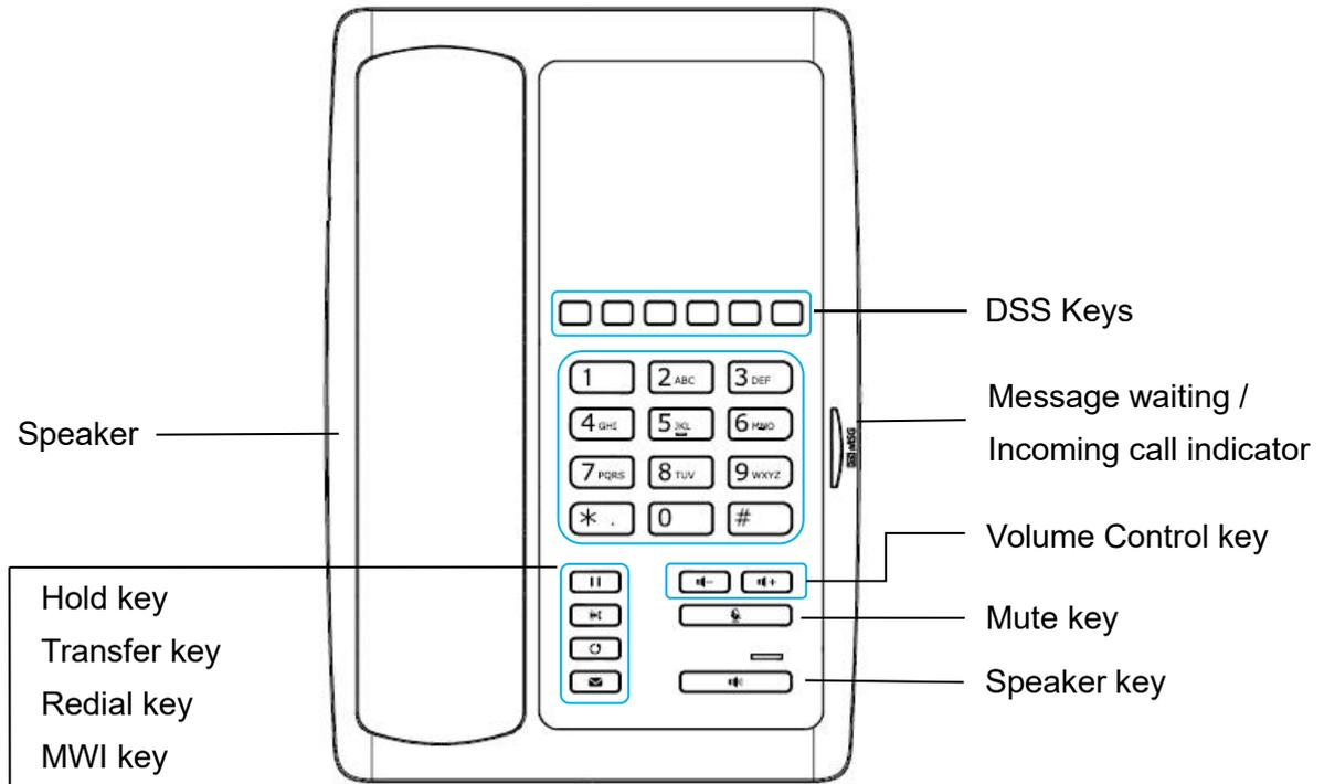
The above picture shows the keypad layout of the device. Each key provides its own specific function. User should refer to the illustration in this section about the usage of each key and the description in this document about each function.
