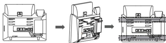
2. Insert the tabs on the wall mount bracket into the slots on the back of IP phone. And then slide the wall mount bracket to right.
