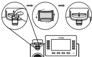
The hookswitch tab has a lip which allows the handset to stay on-hook when the IP phone is mounted vertically.
