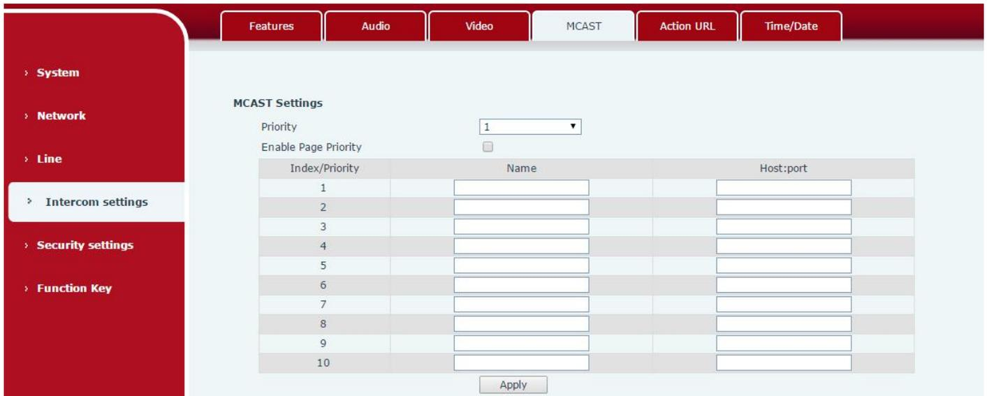
It is easy and convenient to use multicast function to send notice to each member of the multicast via setting the multicast key on the device and sending multicast RTP stream to pre-configured multicast address. By configuring monitoring multicast address on the device, the device monitors and plays the RTP stream which sent by the multicast address.
