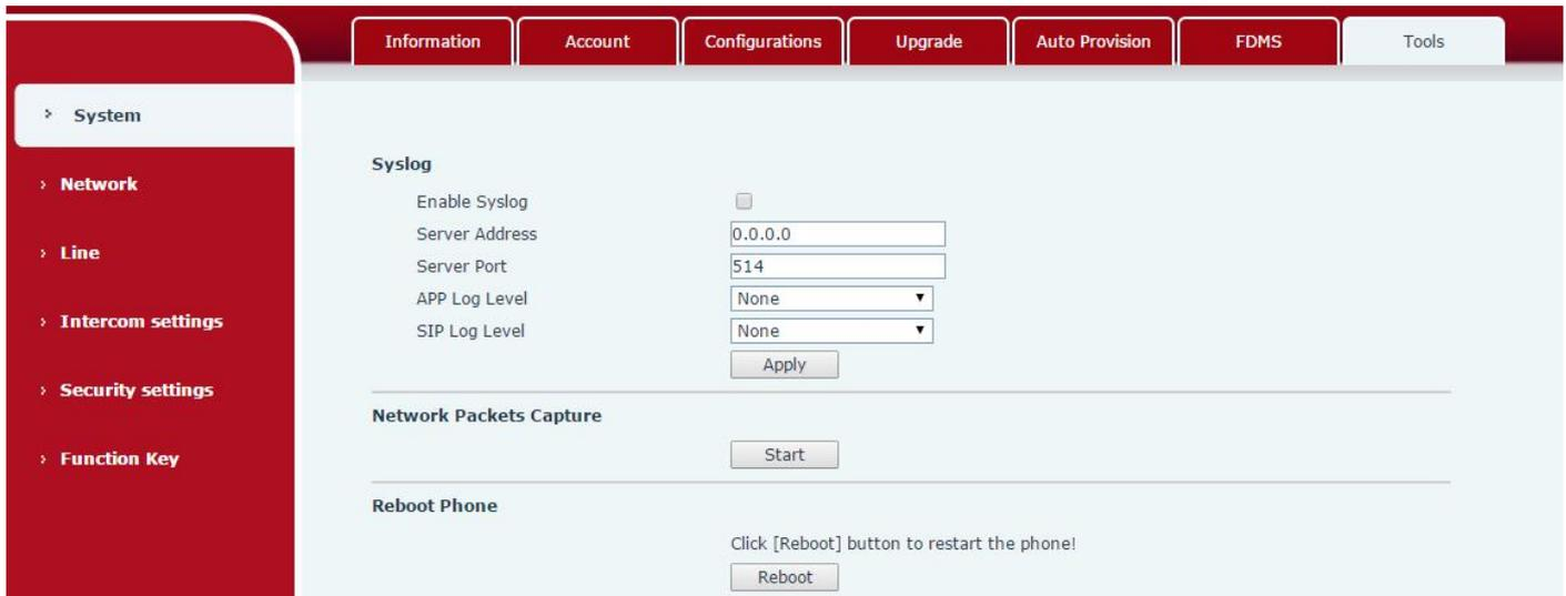
Syslog is a protocol used to record log messages using a client/server mechanism. The Syslog server receives the messages from clients, and classifies them based on priority and type. Then these messages would be written into a log by rules which the administrator has configured.
