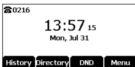
The idle screen displays the label of the current account, time and date, and four soft keys.
