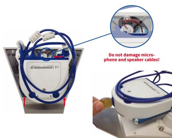
Do not damage microphone and speaker cables!
