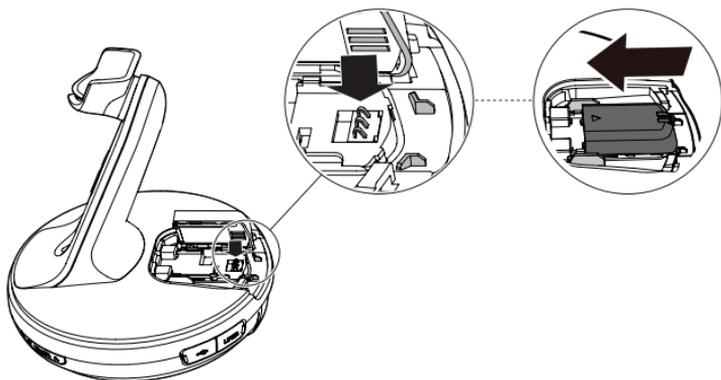
7. Slide the battery compartment cover back to the headset base.
