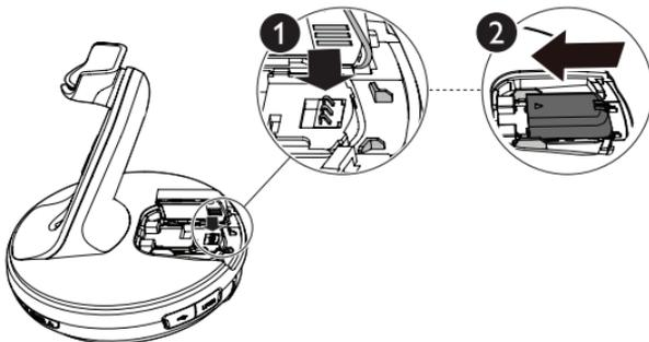
3. Slide the battery compartment cover back to the headset base.
