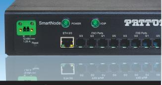
The SmartNode 4140E Series of VoIP Media Gateways supports up to eight telephones integrating PSTN, PBX, and standard phones for voice and fax over any IP network. The corporate, small, or remote office can use voice-over-packet services to eliminate toll charges, access local PSTN calling, and secure voice traffic. Now ruggedized to handle the extreme environmental conditions your application calls for.
