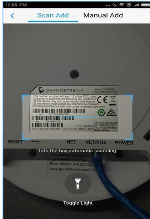
**Figure 7 : Adding New AP by Scanning the Barcode**
