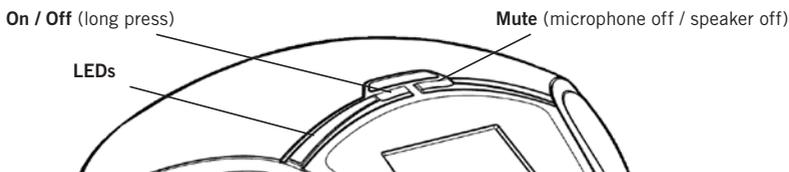
With a computer connection, the LEDs first light up when a communication program that uses the microphone starts.
