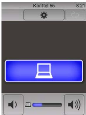
The computer normally only activates the speaker in the Konftel 55 if there is no other program running that can use the microphone. This means that the Konftel 55 acts as a computer speaker and that the audio processing in OmniSound® is turned off so that the sound is not altered.
