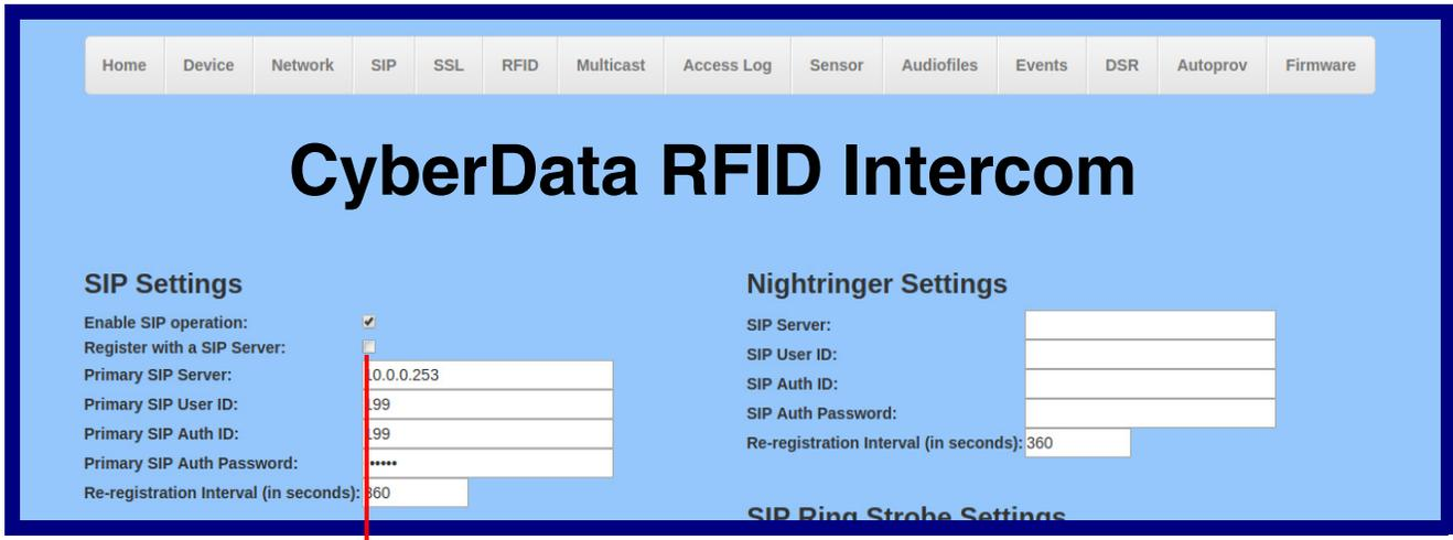
Device is set to NOT register with a SIP server
