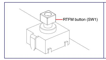
When the device is operational and linked to a network, you can use the Reset Test Function Management (RTFM) button (SW1) to restore the device to the factory default settings.
