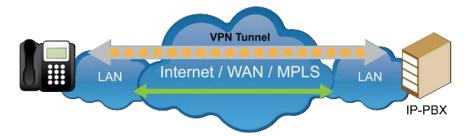
In this example, the IP-PBX resides behind a Firewall, the Firewall is the border element between Internet or Untrusted Network Zones and Local Area Networks or Trusted Zones. The Firewall is a network security device and will forward the VPN (IPSec) traffic from the Remote Phone to the IP-PBX.
