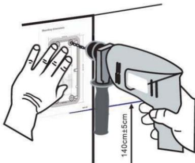
Figure 3-3 Wall Mounting / Built-in
