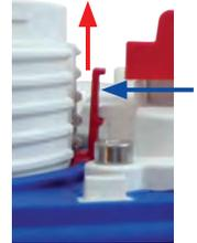
3. **Remove the sensor module cable from the sensor or blind module:** The sensor module cables are secured using a special cable lock with bayonet catch. To remove the bayonet catch turn it counter-clockwise until it gently snaps open. Take off the catch and pull out the cable.
