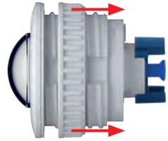
2. **Remove the transport plugs:** Gently pull the two transport plugs out of the sensor module sockets by lifting the rim of the plugs. Now pull the connectors of the sensor module cables out of the back of the transport plugs; take care not to damage the connectors or the cables. **Make sure that you do not pull the sensor module cables out of the housing!**
