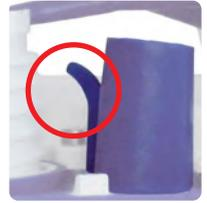
3. Push the front element into the housing and make sure that the sensor module cable remains under the retaining lug (red circle in detail image).
