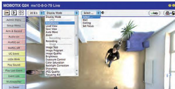
As a result, you will get a **perspective-corrected panorama view** for each image sensor matching the specified installation position. Panorama view is configured as the factory setting and it can be changed as described below.
