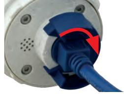
7. **Insert the sensor module:** Make sure that the MOBOTIX lettering on the sensor module is at the “9 o’clock” position as shown in the figure. Using the black module wrench, turn the sensor module clockwise until it stops.
