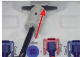
In order to ensure the weatherproofness of the M16, make sure that you only use genuine MOBOTIX patch cables!
