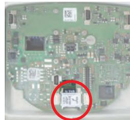
5. **Unlock MicroSD card:** *Carefully* slide the metal latch to the right (using your fingernail).
