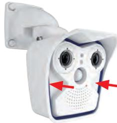
5. Using the supplied 5 mm Allen wrench, tighten the two bolts at the back of the camera housing. Push the two rubber plugs back into the opening of the screws to prevent humidity and dirt from entering the camera.
