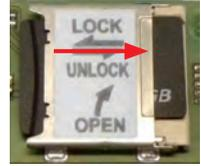
6. **Remove the MicroSD card:** Lift the metal latch upwards and to the right and remove the SD card.
