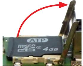
7. **Insert and lock the MicroSD card:** Insert the MicroSD card and close the metal latch. Gently slide the metal latch (using your fingernail) back to the left to lock the MicroSD card.
