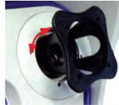
3. If required, clean the inside of the protective glass lens using a clean, lint-free cotton cloth.
