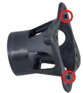
4. **Remove the sensor or blind module:** Set the black module wrench onto the sensor or blind module, so that the two notches lock into the two holes of the module (at the 12 and 6 o'clock positions). Turn module wrench counter-clockwise by 90 degrees until it stops.
