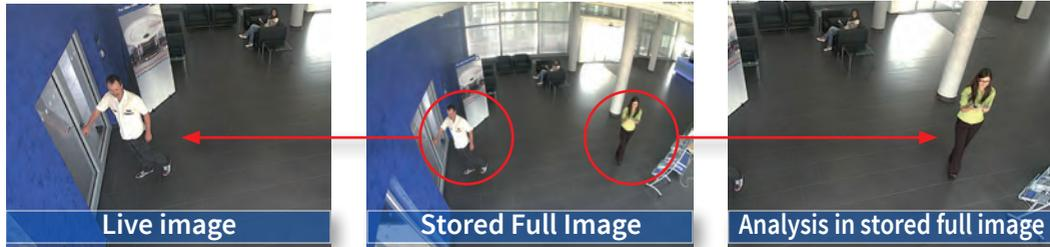
This means that you can use the vPTZ features in VGA image size to pan, tilt and zoom in the live image while the camera is, for example, recording full images at 1 fps in MEGA or 6MP image size.
