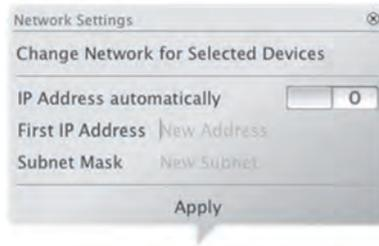
If you have assigned a fixed IP address to your computer, you will certainly prefer to assign fixed IP addresses to the cameras. To do so, enter the IP address and the subnet mask. The IP address is incremented automatically for each selected camera.
