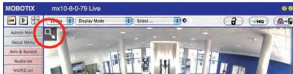
4. Using the **OnScreen Control** visible in the live camera image, you can now change the displayed live camera image as desired (panning, tilting, zooming, rotating and panorama correction). See figure on the right. When doing so, the vPTZ function using the mouse or joystick is deactivated. In case of a M16 with two sensor modules, click the corresponding camera image (right/left) to edit it (highlighted with a yellow frame).
