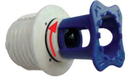
6. Adjust the image sharpness according to the live image on a computer monitor. Use the blue lens wrench for this purpose and turn the lens cautiously to the left and to the right. ***Do not turn the lens too far or with force to avoid damaging the image sensor!***
