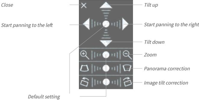
To use the OnScreen Control, click the arrows in the top area for shifting the image section. In the bottom areas, which are displayed when needed, click to the left and/or right of the center point.
