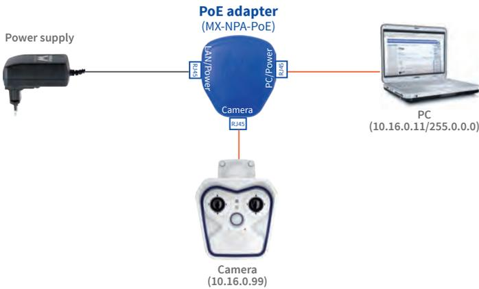
The PoE adapter replaces the crossover cable when directly connecting to a computer
