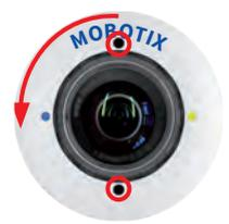
Push the sensor or blind module out of its socket.
