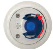
6. **Connect the sensor module cable to the sensor module:** Guide the cable through the opening in the front element and firmly push the sensor module cable into the connector. Apply bayonet catch as shown and turn it clockwise until it gently snaps shut.
