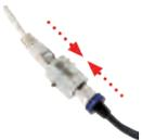
4. **Connect the cable:** Connect the on-site network cable to the camera patch cable using an adapter or insert the patch cable into the RJ45 outlet. Take note of the installation manual included in the package when using a MX-Patch-Box. All manuals can be downloaded and printed (as PDF files) from the MOBOTIX website ([www.mobotix.com](http://www.mobotix.com)) in the **Support > Download Center > Documentation > Manuals** section. Make sure that the cables are not bent or squashed.
