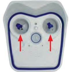
3. **Connect sensor module cable:** Firmly push the sensor module cable into the module's connector as shown in the figure.
