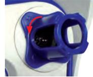
2. If required, clean the inside of the filter using a clean, lint-free cotton cloth.
