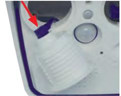
4. **Lock sensor module cable:** Apply bayonet catch as shown and turn it clockwise until it gently snaps shut.
