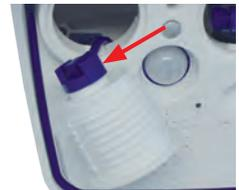
5. **Insert the sensor module:** Make sure that the MOBOTIX lettering on the sensor module is at the "9 o'clock" position as shown in the figure.
