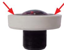
5. Screw the lens with the sealing ring back into the sensor module using the blue lens wrench.
