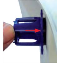
5. Adjust the **polarization filter** according to the camera's live image on the computer monitor. Rotate the filter to the left using the blue lens wrench until you reach the desired setting (maximum 180°).
