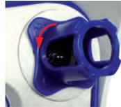
2. Adjust the image sharpness according to the camera's live image on the computer monitor. To do so, position the black module wrench (with the ring-pattern side) on the lens and carefully rotate to the right or left. **Do not turn the lens too far or with force to avoid damaging the image sensor.**
