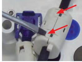
4. **Attach ferrite at the new patch cable:** Attach the hinged ferrite at the new patch cable, leaving a space of exactly 70 mm/2.8 in between the sealing of the plug and the ferrite.
