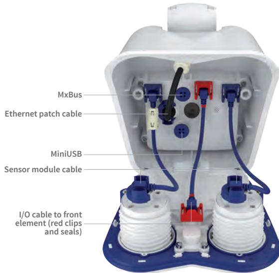
Only use cables with **angled plugs** inside the housing of the M16 (exceptions: patch cables, MxBus connection wires)!
