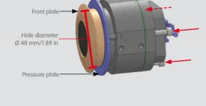
Tighten the cylinder head screws (red arrows) to push the pressure plate against the wall/faceplate Hole diameter Ø 48 mm/1.89 in Possible thickness of wall/faceplate: 0 to 14 mm/0 to 0.6 in
