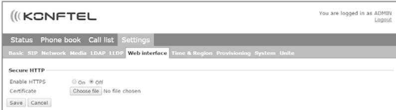
The web server in the Konftel 300IPx supports secure connections using HTTPS.
