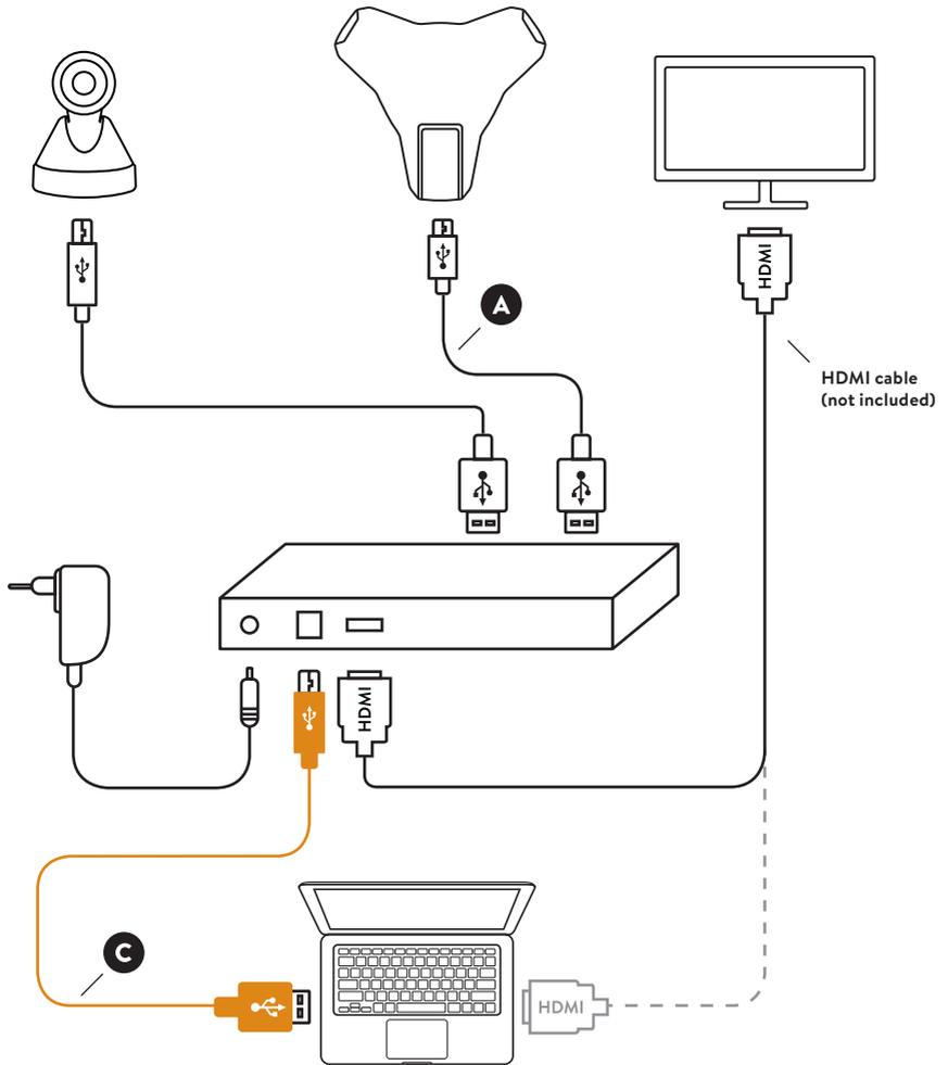
ⓘ Before connecting the USB cable **C** to the laptop, make sure that the DisplayLink driver is installed on the laptop.
