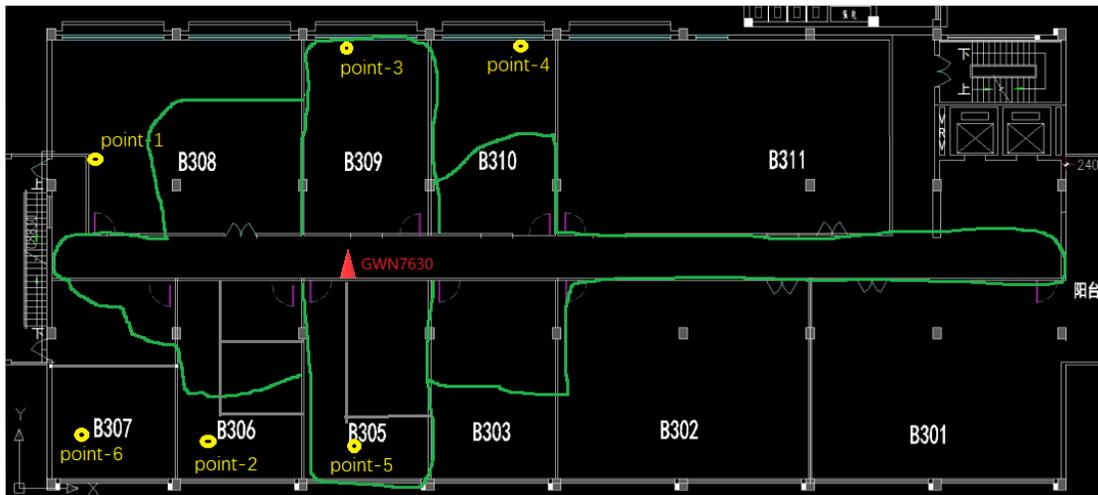
**Figure 4: CAP Direct wall-through coverage**
