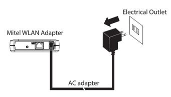
While reconnecting the AC plug to the outlet, press and hold the push switch at the front of the Mitel WLAN Adapter. Keep pressing and the factory default configuration will begin.
