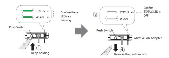
The Mitel WLAN Adapter will start to communicate with your wireless router.
