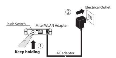
When the WLAN LED turns from Green to Red, release the switch. The factory default configuration is completed. After the factory default configuration is completed, the Mitel WLAN Adapter will restart.
