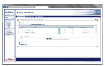
\* If the destination network is not displayed in the Wireless Network List, click Detailed Configuration at the top of the page. In the page displayed, enter the wireless settings of the network that you wish to connect Mitel WLAN Adapter to, and click the Submit button. Refer to the HELP for details on each setting.
