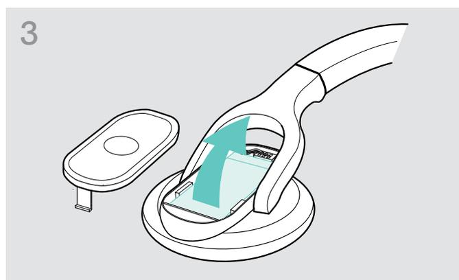
▷ Remove the rechargeable battery and carefully loosen the connector plug of the rechargeable battery.
