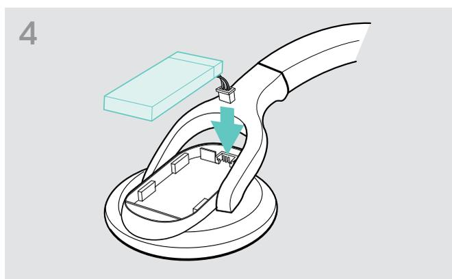
▷ Insert the connector plug of the new rechargeable battery into the connection socket. Observe correct orientation of the connector plug.
