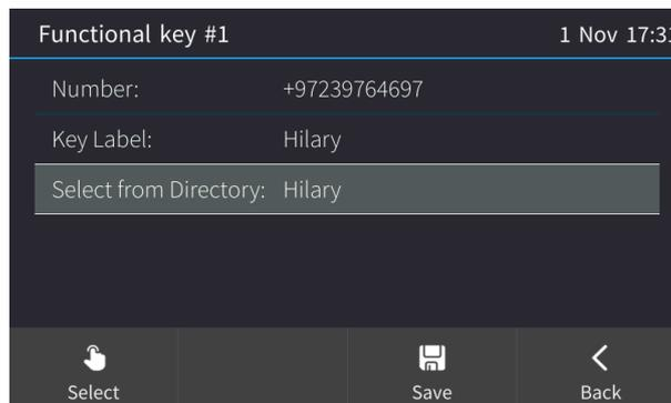
4. Touch the **Save** softkey; the touch screen reverts to idle mode displaying the name of the contact you configured ('Hilary', in this example):
