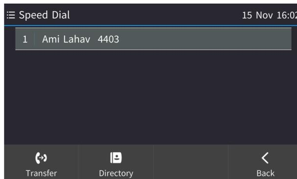
3. In the Speed Dial screen that opens, select the Speed Dial of the contact to transfer the call to.
