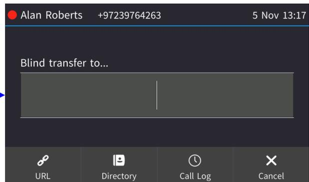
2. In the 'Blind transfer to' field, enter Hilary's number (4697) and then touch the **Transfer** softkey or wait; Hilary's AC-HRS device rings.
