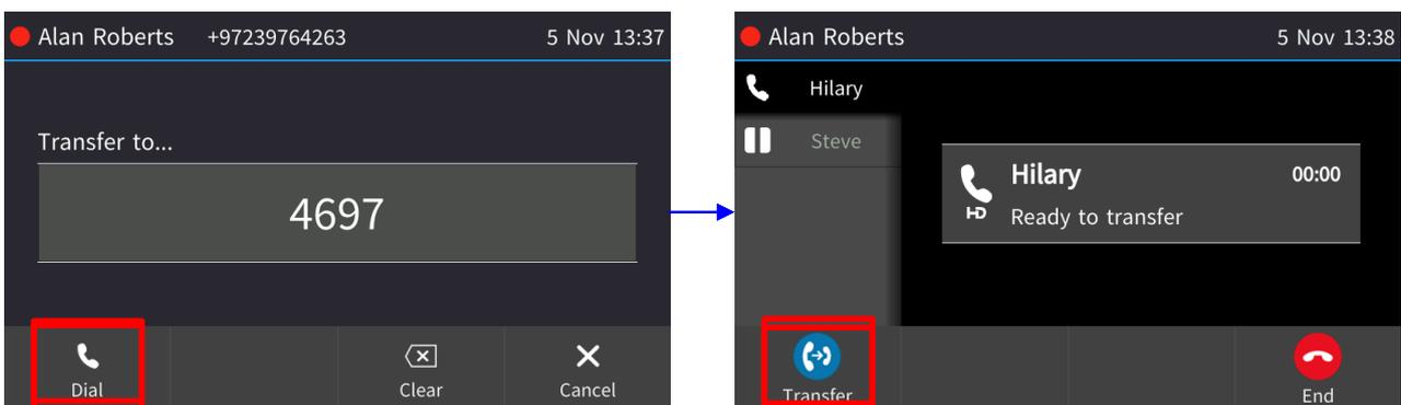
4. Touch **Transfer** or press the TRANSFER key on the AC-HRS. Hilary is connected to Steve.
