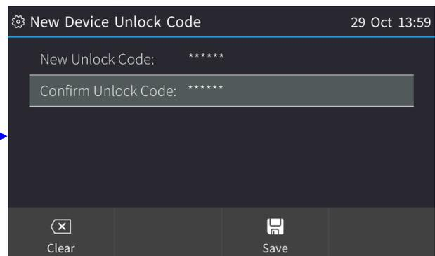
3. Enter the new unlock code, scroll down and re-enter it, and then touch the **Save** softkey; if left inactive for 10 minutes (default) and if the lock feature is enabled (see below), the phone will automatically lock.
