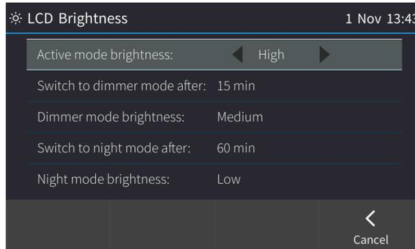
2. Touch an option and then press the navigation control's left or right rim to navigate to the brightness level that suits you best. Use the table below as reference.
