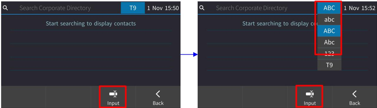
3. If you're searching for **Alex** (for example), on the dialpad press once the **2** key, press three times the **5** key, press twice the **3** key, and if necessary, press twice the **9** key.
