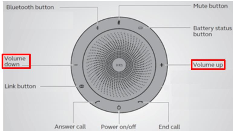
Here's how to adjust the volume on the UC-HRS-458-SPK. Use the figure as reference.
