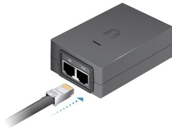
4. Connect an Ethernet cable from your LAN to the **LAN** port on the *PoE Adapter*.
