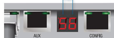
**Note:** If the LED Display indicates an overload condition **OB**, see **"RX Gain" on page 30** for more details about *RX Gain* and overload condition.
