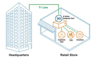
Sangoma telephony cards integrate into most commercial grade appliances and transmit in-store data to headquarters over a T1 connection, using WAN protocols
