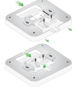
Note: To unlock the access point, push the locking tab toward the ceiling and slide the access point out of the bracket.
