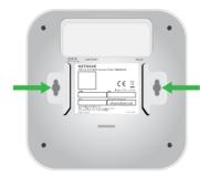
Mark the wall where you want to insert the provided anchors and screws, which must be 3.875 in. (98.5 mm) apart, and insert the anchors and screws.
