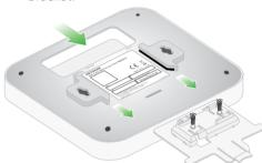
Slide the access point into the bracket until it locks in place. The locking tab must be at the front of the access point.
