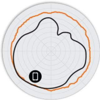
Figure 3. R510 5GHz Azimuth Antenna Patterns
