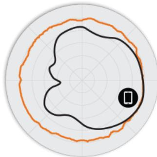
Figure 4. R510 2.4GHz Elevation Antenna Patterns
