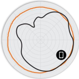
Figure 3. R610 5GHz Azimuth Antenna Patterns
