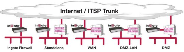
QoS (voice quality over data-crowded accesses) is provided by the SIParator. DMZ-LAN & DMZ modes also require QoS setup in existing firewall.
