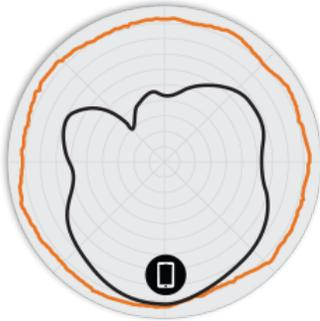
Figure 3. R710 5GHz Azimuth Antenna Patterns
