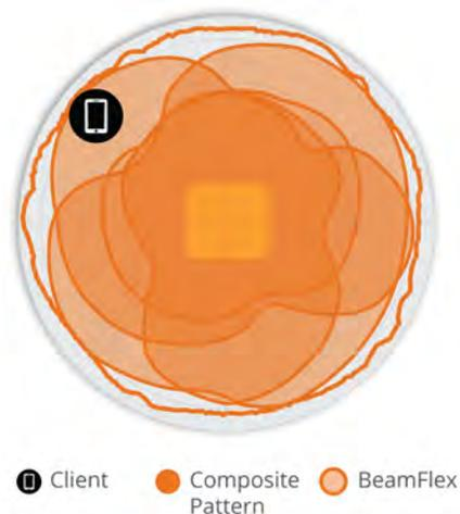
Figure 2. R350 2.4GHz Azimuth Antenna Patterns
