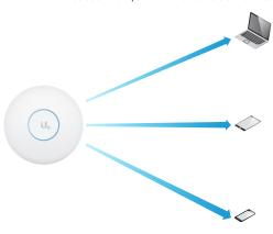
MU-MIMO with 2x2 and 1x1 clients: The UniFi AC SHD AP communicates with one 2x2 client and two 1x1 clients at a time.
